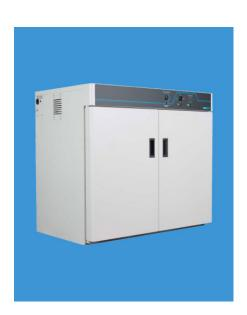
This design does not require blowers or fans within the incubator chamber where samples are susceptible to cross contamination and the drying effects of convection. Five strategically placed heating elements, including a heated outer door, ensure uniform heating even when the incubator chamber is fully loaded.
