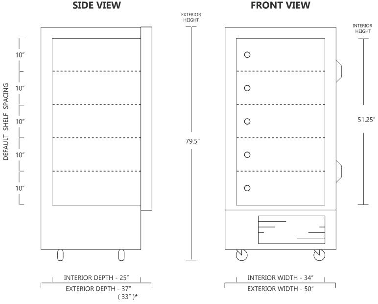
\*TO PASS THROUGH DOORWAYS, THE DOOR CAN OPEN A FULL 180°, TO REDUCE THE UNIT EXTERIOR DEPTH TO 33"
