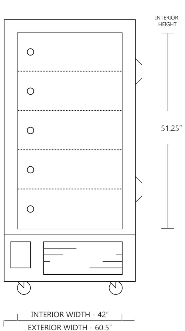
\*TO PASS THROUGH DOORWAYS, THE DOOR CAN OPEN A FULL 180°, TO REDUCE THE UNIT EXTERIOR DEPTH TO 33"
