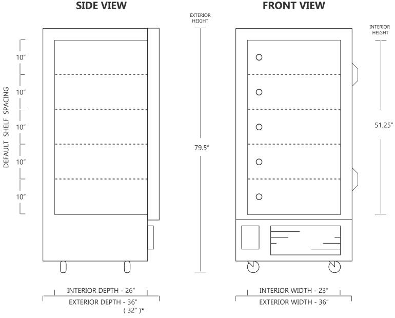
\*TO PASS THROUGH DOORWAYS, THE DOOR CAN OPEN A FULL 180°, TO REDUCE THE UNIT EXTERIOR DEPTH TO 32"
