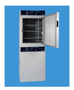
This design does not require blowers or fans within the incubator chamber where samples are susceptible to cross contamination and the drying effects of convection. Five strategically placed heating elements, including a heated outer door, ensure uniform heating even when the incubator chamber is fully loaded.
