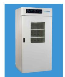
Our unique forced air circulation system creates a one-pass circulation pattern that provides both exceptional temperature uniformity and rapid heat recovery. The chamber floors are ruggedly reinforced to support roller apparatus or shakers. The SMI31 is supplied with six sturdy shelves that will not sag or bend under heavy loads.
