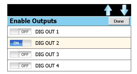
For example, if digital output 2 is used as a control output to turn on a circulating fans that are common to both system A and system B when a system event is turned on, then select digital output 2 from the list. This will enable the redundancy logic whenever the circulating fans are on. Additional outputs can be selected if necessary. Once all selections have been made, press the 'Done' button to accept the output selections and return to the Redundancy Setup screen.
