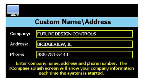
To edit the company, address and phone number, press the desired field and enter the desired text. Each field can be entered with a maximum of 24 characters that will be displayed on the splash screen when the nCompass starts.
