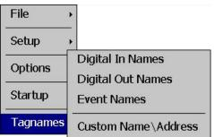
The **Tagnames** menu provides access to the text editing functions of the configurator which allow the event and digital input and output names to be changed to match their use in the system. The menu also provides access to edit the splash screen information that is shown when the system starts.
