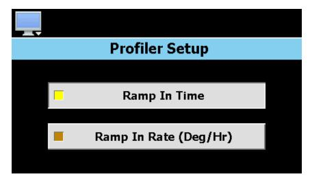
When **Ramp In Time** is selected, the steps of the profile are entered as units of time in hours, minutes and seconds with individual set points for each control loop in the system. When the steps of the profile are executed, the profiler will ramp the set points of each loop individually to the set point of the step, linearly over the time duration of the step.
