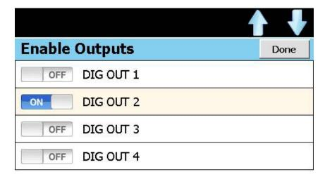
For example, if digital output 2 is used as the control output for the refrigeration system when a system event is turned on, then select digital output 2 from the list. This will enable the defrost logic whenever the refrigeration system is on. Additional outputs can be selected if necessary. Once all selections have been made, press the 'Done' button to accept the output selections and return to the Defrost Setup screen.
