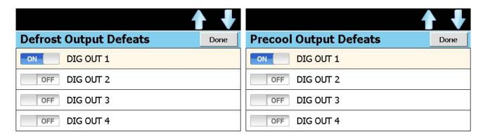
For example, if digital output 1 is used as the control output for the system fans when a system event is turned on, then select digital output 1 from the list. This will turn off the fans during defrost and precool whenever the defrost cycle actives. Additional outputs can be selected if necessary. Once all selections have been made, press the 'Done' button to accept the defeat selections and return to the Defrost Setup screen.
