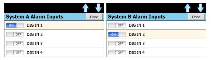
For example, if digital input 1 will be used for the system A failure input, then select digital input 1 from the list. If digital input 2 will be used for the system B failure input, select it as the alarm input for system B. Additional inputs can be selected if necessary. Once all selections have been made, press the 'Done' button to accept the input selections and return to the Redundancy Setup screen.
