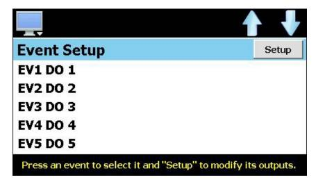
To assign outputs to an event, touch the desired event in the list box and press the 'Setup' button. The 'System Event Output Configuration' screen will then be shown.
