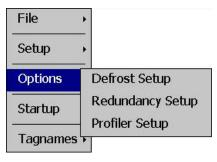
The **Options** menu provides access to additional controller options including the setup of defrost and redundancy operation as well as the profiler mode of operation.
