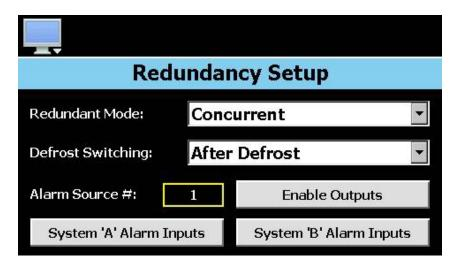
The **Redundant Mode** selection is used to choose how redundancy operates. Available selections are Disabled, Concurrent and Alternating. The concurrent and alternating redundancy modes select the back-up system mode of operation. When concurrent is selected, both system A and system B will operate at the same time when the selected alarm source in is alarm. When alternating is selected, nCompass will switch to the back-up system on alarm.
