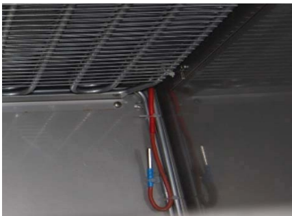
Mounting of the sensor in the freezer
