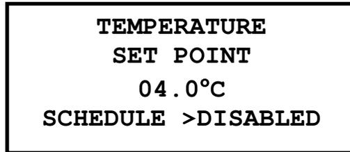
Press the **ENT** key until the cursor moves to the schedule field. Use the Up or Down arrow key to enable the schedule. Press the **ENT** key and the first of 21 Ramp and Soak screens will be displayed.
