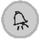
**ALARM KEY:** Displays active alarms, alarm history, acknowledge alarms, and clear alarms. Back lit when an alarm is active.
