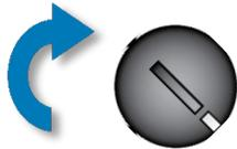
**2. Turn the dial counterclockwise until the Over Temperature Activated light illuminates.**
