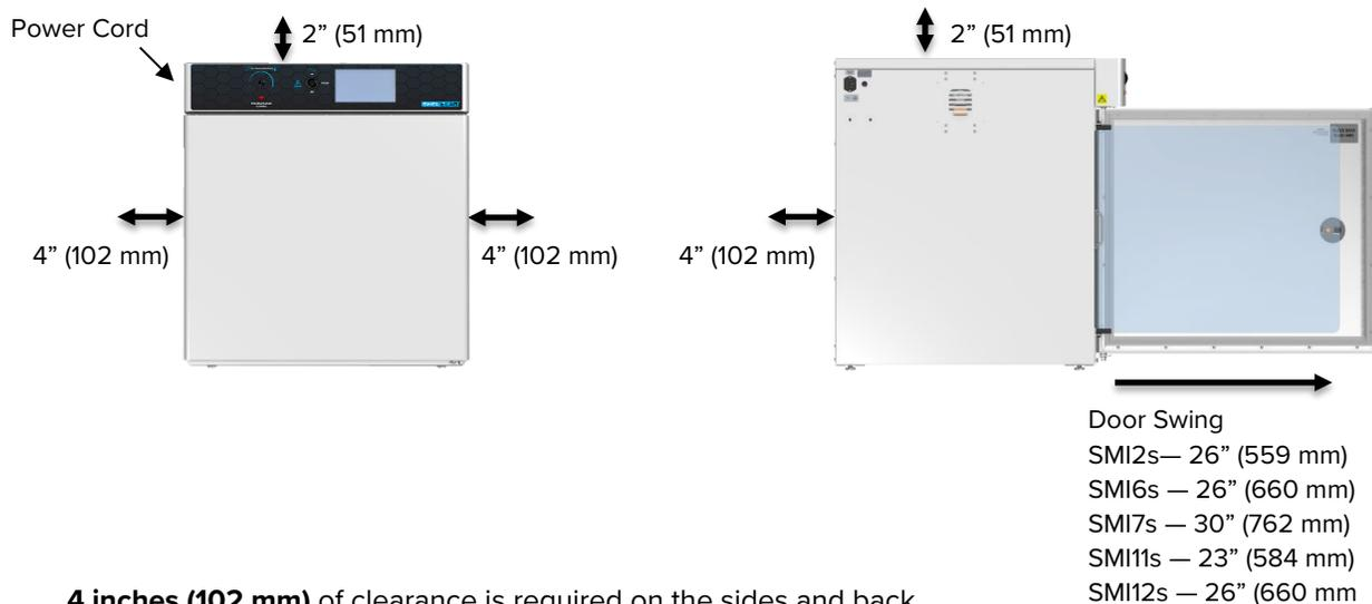
**4 inches (102 mm)** of clearance is required on the sides and back.
