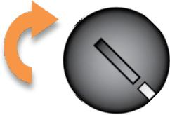
**Before starting this procedure, turn the OTL dial clockwise to its maximum setting, if not already set at max.** This prevents the heating cutoff system from interfering with this procedure.
